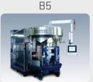
The Applied HCT B5 wafering system cuts both monocrystalline and multicrystalline silicon stock into ultra-thin wafers. The system provides best in class process yield with the industry's highest productivity, and is a proven platform for advanced wire technologies.
