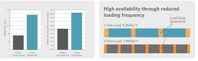
At industry leading 120µm wire size and 180µm wafer thickness, the B5 load advantage delivers >15% higher productivity per system when compared with conventional 1m load tools. When combined with the B5 25% footprint advantage over these same tools, the productivity advantage for a given factory size approaches 50% more wafers per year.
