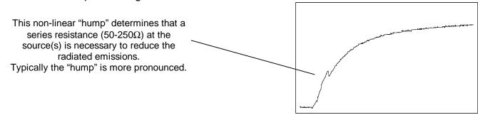
Values of the resistance will depend on the speed and the current of the devices, it may be best to place 0Ω jumpers at the source(s) to allow changing of the values once the board is created.
