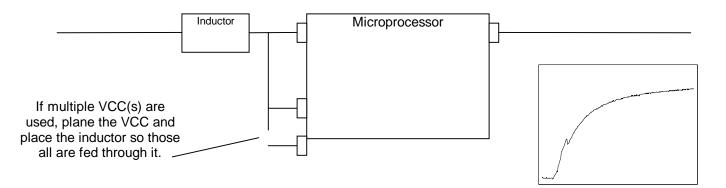
Capacitance (.1uF to .001uF) is recommended for microprocessors, which do not have the "hump" characteristic on the outputs. Be sure to place the capacitor at the microprocessor and reference it to the ground plane of the microprocessor with a short and fat (low inductance) trace.
