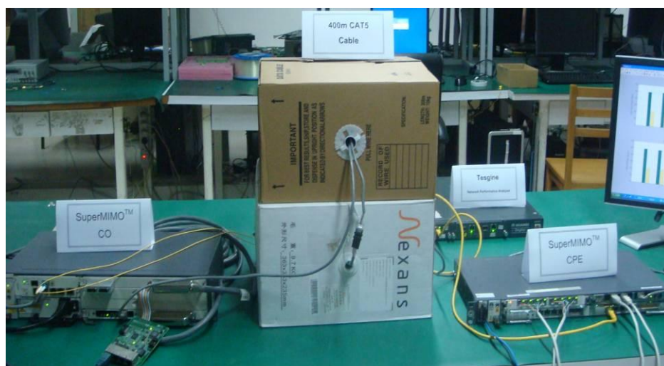
Figure 2-9 Test configuration for the SuperMIMO prototype
