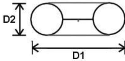
$$C = 2.8 \times \left( 1.2781 - \frac{D2}{D1} \right) \times \sqrt{\frac{2 \times \text{PI}^2 \times (D1 - D2) \times \left( \frac{D2}{2} \right)}{4 \times \text{PI}}}$$
