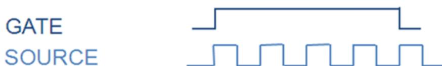
$$\text{待测信号频率} = \text{计数值} / \text{计数时间}$$
