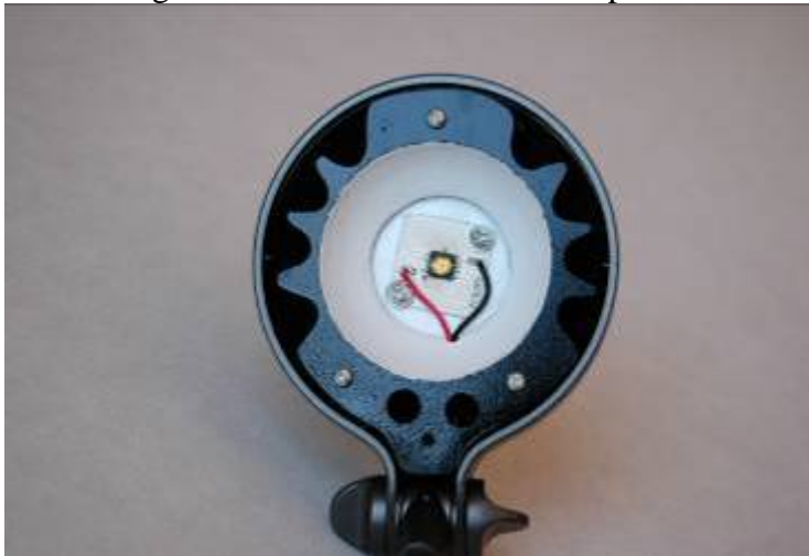
Figure 5: Cree MC-E mounted on sub-mount and connected to heatsink
