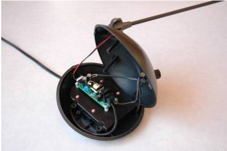
Figure 7: NCP1014LEDGTGEVB constant current driver board mounted in base of desk lamp
