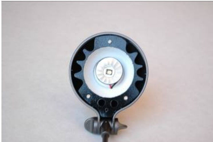
Figure 5a: Cree MC-E including reflector optic
