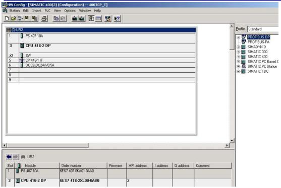
For CP443-1 module we need to define the IP address and subnet mask.
