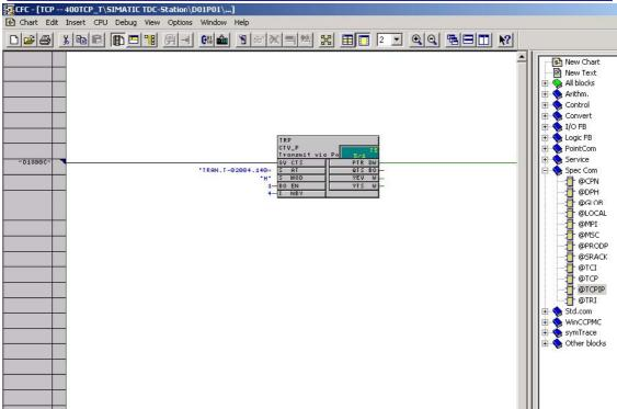
2.2.4 Insert the DWR\_D block to write the communication content to the communication buffer
