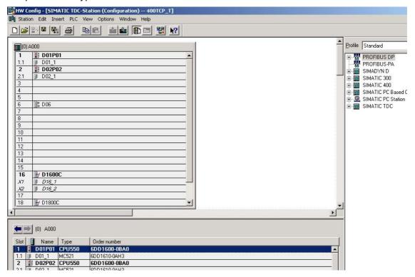
2.1.5 Define the CPU module and communication module properties
