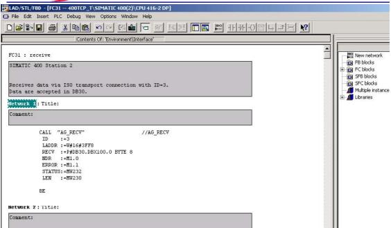
Because we use DB30 and DB31 in the program FC30 and FC 31, we must insert these two data block and download it to the CPU.
