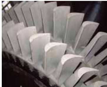
图 7 再制造后叶片及组装后转子 Fig.7 The blade and assembled rotor treated with laser remanufacturing
