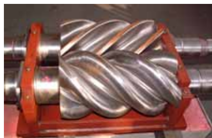
图 14 激光再制造后的转子副 Fig.14 The male and female rotors processed with laser remanufacturing
