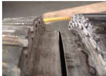
图 5 轮盘损伤状态 Fig.5 Damaged rotary table
