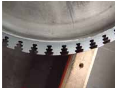
图 8 激光再制造后的烟机轮盘 Fig.8 The rotary table of flue gas turbine processed with laser remanufacturing
