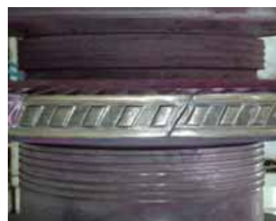
图 12 激光再制造后的围带铆钉 Fig.12 the rivet processed with laser remanufacturing
