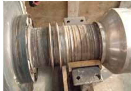
图 9 激光再制造后的主轴径 Fig.9 The axis processed with laser remanufacturing
