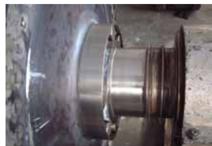
图 6 主轴径及气封损伤状态 Fig.6 Damaged axis and gas seal
