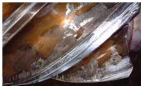
图 13 转子工作面损伤状态 Fig.13 Damaged rotor working face
