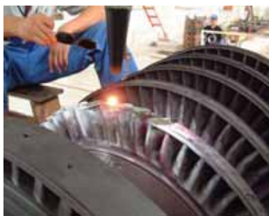
图 11 围带铆钉激光熔覆中 Fig.11 The rivet being processed with laser cladding
