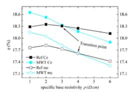
**Figure 5**: 2D "Sentaurus Device" simulation of a MWT and conventional solar cell [25]. The simulation shows a transition point depending on the bulk lifetime (mc, Cz) and base resistivity. Boron-oxygen induced degradation effects of the bulk lifetime are not regarded. The absolute values for the bulk lifetime are based on estimated input parameters, so especially for mc-Si an overestimation is probable.
