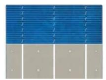
**Figure 4:** Picture of the front and rear of a typical mc-MWT solar cell (156x156 mm<sup>2</sup>) with three continuous rear busbars processed at Fraunhofer ISE [24].
