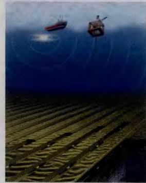
图7 光纤声波检测器的海底铺设效果图 Fig. 7 Fiber optic permanent seismic monitoring installation, covering the reservoir area of interest
