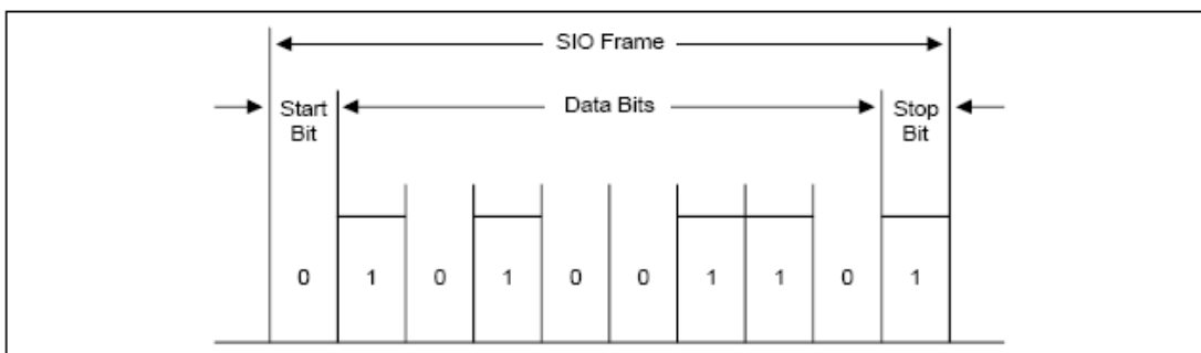
Figure 11-4. Serial I/O Frame Timing Diagram (Normal UART)
